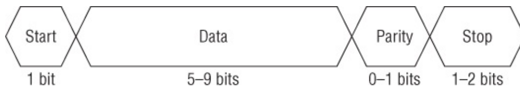
Figure 5.3 A serial packet containing data
